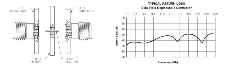
Although Johnson Components<sup>™</sup> does not publish a VSWR specification for field replaceable connectors, typical connector VSWR can be expected to be less than 1.1 + .01f (f in GHz). A VSWR specification is not stated because an industry standard method for tes ting field replaceable connectors does not exist. The actual performance of the connector is dependent upon the application for the following reasons:
