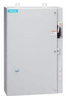
Non-reversing motor starter, Size 3, Three phase full voltage, Solid-state overload relay, OLR amp range 25-100A, 240V 50Hz / 277V 60Hz coil, Combination type, 100A fusible disconnect, 100A/250V fuse clip, Enclosure NEMA type 4/12, Water/dust tight for outdoors, Extra-wide enclosure
