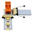
Peel back adhesive and insert LED strip between black latch and bridge. Be sure polarities are matched.
