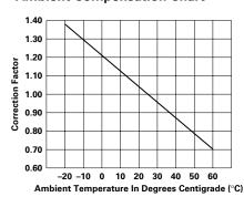
To use this chart: Read up from the ambient temperature to the curve, and across to find a correction factor. Multiply the breaker rating by the correction factor to determine the compensated rating. Calculate the overloads in terms of the compensated rating to use the published trip curve. Do not use these devices outside their specified operating temperature ranges.
