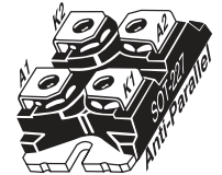
SOT-227[J] Antiparallel Configuration (Isolated Base)
