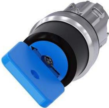
Key-operated switch O.M.R, 22 mm, round, metal, shiny, lock number 73038, blue, with 2 keys, 2 switch positions O-I, latching, actuating angle 90°, 10:30h/13:30h, key removal O, with laser labeling, upper case
