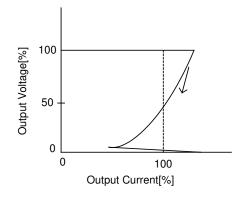
Note) A drooping characteristic may be seen in the over current protection state as shown on the left figure. Note that output voltage may not go up if connected to a nonlinear load such as a lamp, motor, etc., or a constant current load.
