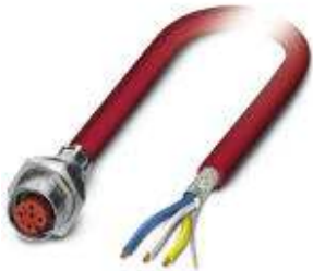
Bus system flush-type socket, CC-Link, 4-pos., M12, SPEEDCON, shielded, rear/screw mounting with Pg9 thread, with 0.5 m bus cable
