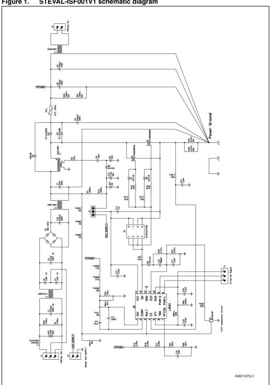
Figure 1. STEVAL-ISF001V1 schematic diagram
