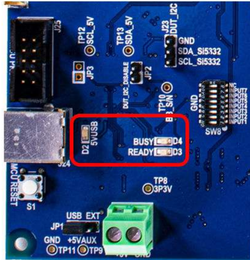
Figure 3.2. Si5332-8A-EVB LED Locations
