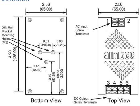
Dimensions: inch (mm) Case Tolerance: ±0.05 (±1.30)
