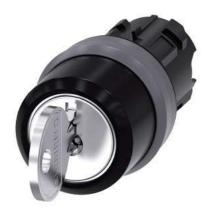
RONIS key-operated switch, 22 mm, round, plastic with metal front ring, lock number SB30, with 2 keys, 3 switch positions I-O<II, left latching, right momentary contact type, actuating angle 2x45°, 10:30h/12h/13:30h, key removal I, possible special locks: SB31, 421, 455, with laser labeling, lower case
