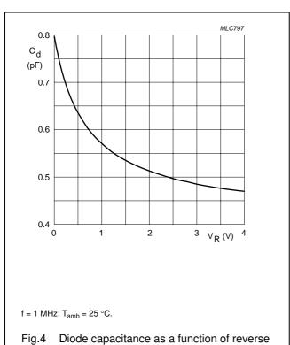
Fig.4 Diode capacitance as a function of reverse voltage; typical values.
