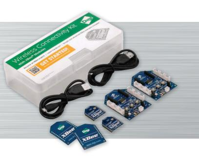
Digi's Wireless Connectivity Kit provides a hands-on way to learn how to use XBee® RF modules for device connectivity and sensor networking.
