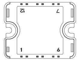
All multiple inputs and outputs must be shorted together 3/4; 5/6; 7/8; 1/2; 9/10
