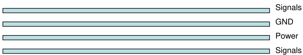
Figure 6: Typical 4-layer PCB construction
