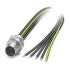
Device connector, rear mounting, Power, 5-position, Socket, M12, coding: K , on free cable end, Rear mounting, M16 x 1.5, Individual wires, cable length: 1.5 m, 2.50 mm<sup>2</sup>, PEX litz wire, Alternative product in accordance with RoHS II without Exemption 6c (Pb <0.1%) item no.: 1238541
