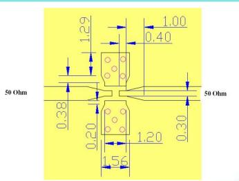
Line width should be designed to match  $50\Omega$  characteristic impedance, depending on PCB material and thickness.
