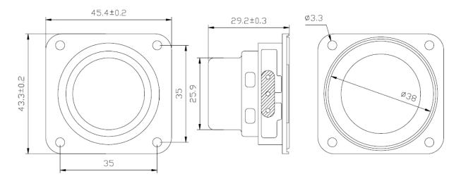
**Note:** Recommended speaker baffle opening is 41mm. Always test-fit prior to closing mechanical design. Please maintain at least 6mm distance between top of frame and next surface.
