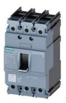
circuit breaker 3VA5 UL frame 125 breaking capacity class S 25kA @ 480 V 3-pole, line protection TM210, FTFM, In=45A overload protection Ir=45A fixed short-circuit protection Ii=10 x In UL489 SB (naval), 50 deg. cel. cable connection on both sides
