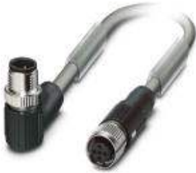
Bus system cable, CANopen®, 5-position, PUR halogen-free, Gray RAL 7001, shielded, Plug angled M12-SPEEDCON, A-coded, on Socket straight M12-SPEEDCON, A-coded, Cable length: 15 m
