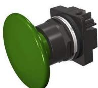
30mm BlackMax, Epoxy Coated Corrosion Resistant Metal Operator, Round Push-Pull Operator Non-Illuminated Mushroom Head Cap Large 2 1/2" (63.5 mm) Plastic, Green 3 Position Pull-Momentary/Push-Maintained UL Listed, CSA Certified NEMA 1,3,3R,4,4X,12,13 & Automotive Standards
