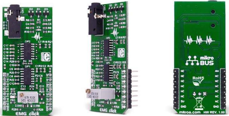
**EMG click** measures the electrical activity produced by the skeletal muscles. It carries MCP609 operational amplifier and MAX6106 micropower voltage reference. EMG click is designed to run on a 5V power supply. The click board™ has an analog output (AN pin).
