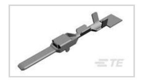
Terminal Type: Tab Mating Tab Width: 2.8 mm [.11 in ] Mating Tab Thickness: .8 mm [.031 in ] Terminal Transmits: 0 – 24 A (Low Power) Wire Size: 22 AWG
