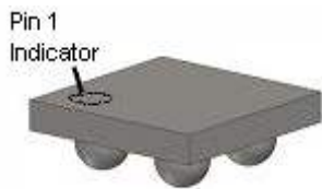
Figure 3. WLCSP Bumps Facing Down (Top View)
