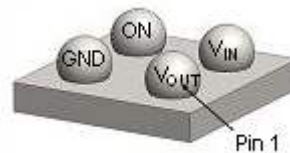
Figure 4. WLCSP Bumps Facing Up (Bottom View)
