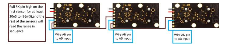
Another recommended chaining method is AN Output Constantly Looping. The first sensor will range, then trigger the next sensor to range and so on for all the sensors in the array. Once the last sensor has ranged, it will trigger the first sensor in the array to range again and will continue this loop indefinitely. Below is a diagram on how to set this up.
