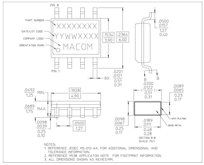
Reference Application Note M538 for lead-free solder reflow recommendations. Plating is 100% matte tin over copper.
