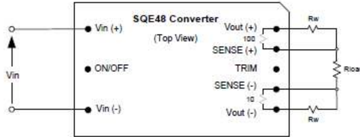
Fig. B: Remote sense circuit configuration
