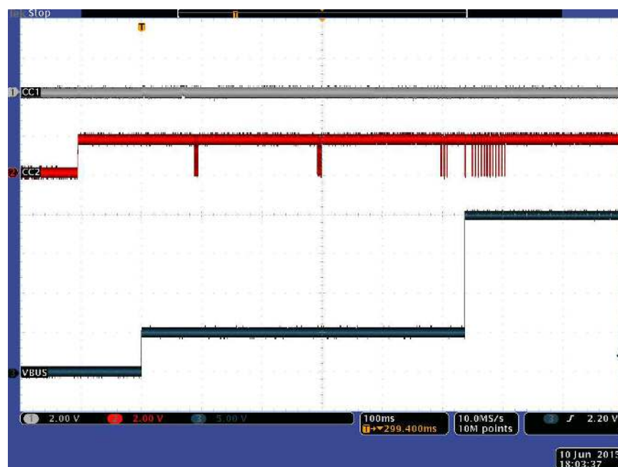
Figure 10. Type-C Connection and PD Negotiation
