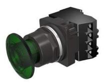
30mm BlackMax, Epoxy Coated Corrosion Resistant Complete Metal Unit Illuminated Twist-to-Release Transformer type, 480V AC LED Lamp Mushroom Head Cap Small 1.79" (45 mm) Plastic Cap, Green 2 Position Maintained, Twist-to-Release with 1 N.O. - 1 N.C. Heavy Duty Contacts, A600/P600 UL Listed, CSA Certified NEMA 1,3,3R,4,4X,12,13 & Automotive Standards
