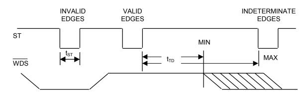
RESET TIMING DIAGRAM—POWER UP Figure 12
