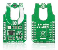
LIN HALL click<sup>™</sup> is a simple solution for adding a linear Hall sensor to your design. It carries an MLX90242 linear Hall sensor IC (with built-in active error correction circuitry) and an MCP3201 12-bit ADC. LIN HALL click<sup>™</sup> communicates with the target board through the **mikroBUS<sup>™</sup>** SPI lines (CS, SCK, MISO). The board is designed to use either a 3.3V or 5V power supply.
