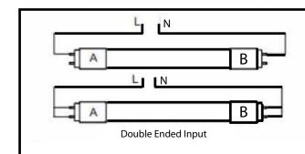
Input voltage: 120-277Vac 50/60Hz
