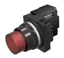
30mm BlackMax, Epoxy Coated Corrosion Resistant Complete Metal Unit Illuminated Indicator Light Full Voltage type, 6V AC/DC Incandescent Lamp, BA9s Plastic Lens, Red UL Listed, CSA Certified NEMA 1,3,3R,4,4X,12,13 & Automotive Standards
