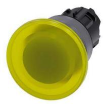
Illuminated mushroom pushbutton, 22 mm, round, plastic with metal front ring, yellow, 40 mm, momentary contact type, with laser labeling, upper case
