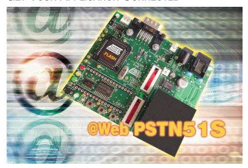
The @Web PSTN51S kit allows the user to evaluate the full range of options available for integrating TCP/IP software into Atmel® C51 Flash Microcontrollers.
