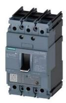
circuit breaker 3VA5 UL frame 125 3-pole, starter protection TM120M, AM, In=90A without overload protection short-circuit protection li=3...7 x In nut keeper kit on both sides
