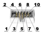
This connector allows programming and debugging via AVR-JTAG or other compatible tools.
