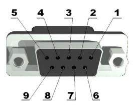
**TXD** Output **Transmit Data.** This is the asynchronous serial data output for the RS232 interface.**RXD** Input **Receive Data.** This is the asynchronous serial data input for the RS232
