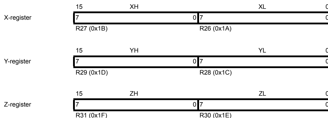
Figure 13-3. The X-, Y-, and Z-registers
