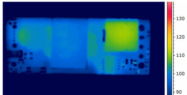
Figure 6. Thermal Image of CPE5C36 (5A output, 70C Ambient, 200lfm airflow, Vin = 48V, airflow from pin 3 to pin 1, T<sub>max</sub> = 109°C)
