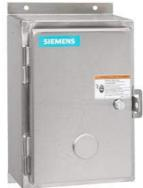
Non-reversing NEMA contactor, Size 0, Three phase full voltage, Contactor amp rating 18A, 3 wire (NO aux included), 110-120/220-240VAC 60Hz coil, Noncombination type, Encl NEMA type 4X 304 S-Steel, Water/dust tight noncorrosive, Standard width enclosure
