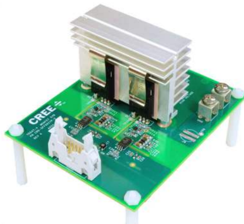
Figure 1. Cree's KIT8020-CRD-5FF0917P-2 evaluation board
