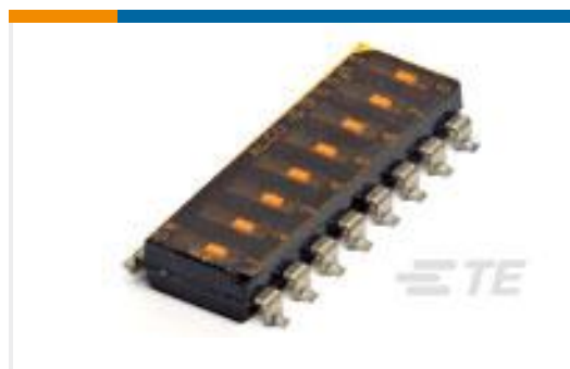
TE Part #1825006-3 GDS02S04=DIP SW,SLIDE,SMT
