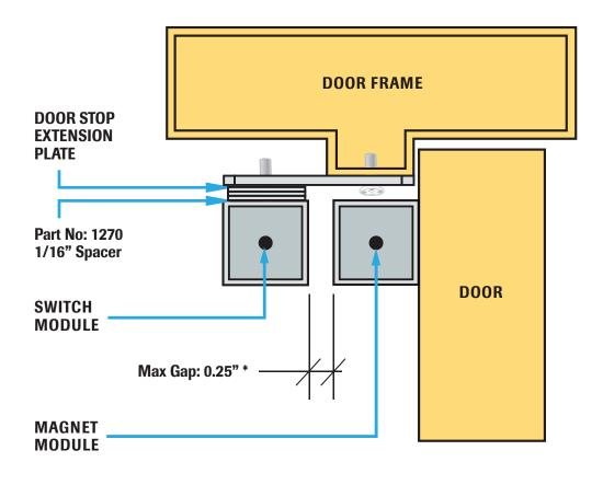
Extension plate is suitable for egress door set-up with a door stop/jam smaller than 2 inches. No plate should be necessary for most door stops which are at least 2 inches thick.
