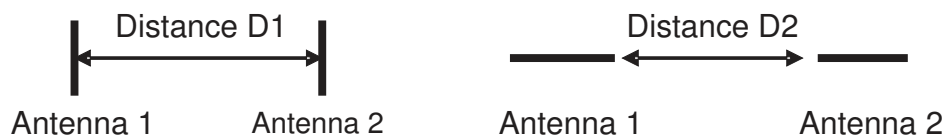
Figure E-1. Distance Between Antennas (Top View)
