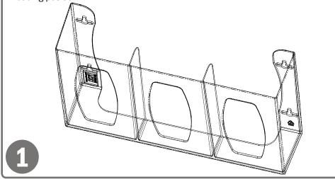
• Mount securely to a wall or cabinet with screws approved and supplied by building maintenance.
