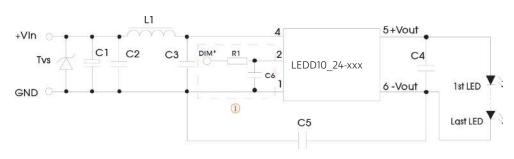
Components Specifications Tvs SMC51A,1500W (ON) L1 CD53-82µH (CEAIYA) C1 470μF/100V (NCC) C2 225K/50V 1210 X7R (TORCH) C3 104K/50V 0805 X7R (TORCH) C4 105K/50V 1210 X7R (TORCH) 102K/2000V 1210 (TDK)) C5 choose or no) 470pF/100V 0805 (TORCH) C6 R1 680Ω 0805 (can be replaced by inductance or magnetic bead)
