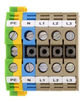
Five-wire mains-connection block, Screw connection, Mounting type:Mounting rail TS 35/7.5 and TS 32, Rated cross-section: 10 mm², Colour: Multi-coloured
