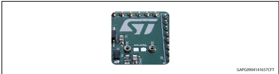
Figure 4: Mounting through-hole sense resistor
