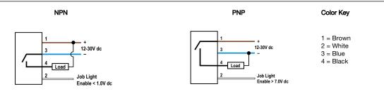
Note: Cabled wiring diagrams are shown. Quick disconnect (QD) wiring diagrams are functionally identical.
